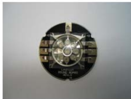
Test set-up on MCPCB
